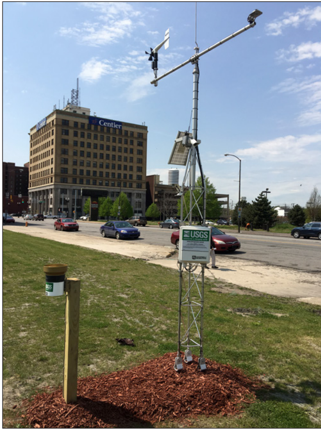
Figure 15. Rain gage and weather station at Gary City Hall study site in Gary, Indiana. Photograph by David C. Lampe, U.S. Geological Survey.
