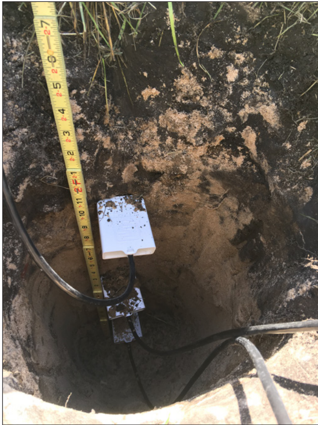
Figure 17. Soil-moisture sensors installed in the wall of an excavation at well CH–2 (413612087201301) at the Gary City Hall study site in Gary, Indiana. Photograph by David C. Lampe, U.S. Geological Survey.
